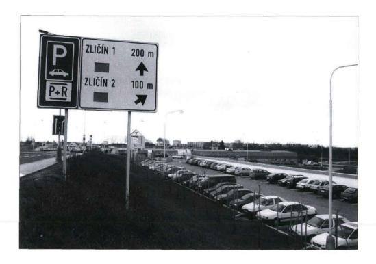
An integral part of an efficient functioning of a P+R system is a vehicle guidance system that provides the drivers the following information: the name of the site, the type of follow-up transport, the current distance from the parking, other P+R sites nearby, the parking occupancy and the follow-up public transport departure times.
