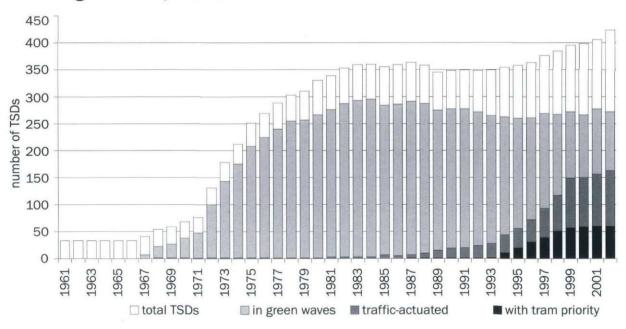
All newly built and reconstructed TSDs are equipped with traffic actuation by vehicle and passenger demand as well as with tram priority. The latter is important especially because the public transport vehicles that share their routes with other traffic are affected with the dense car traffic.
