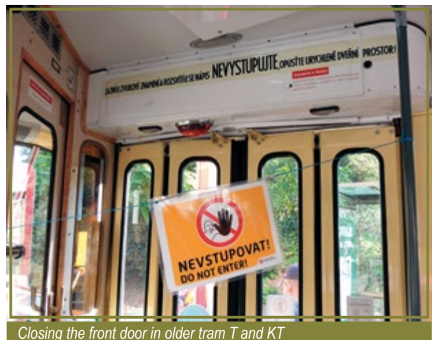
Closing the front door in older tram T and KT
