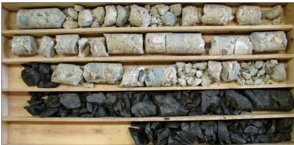
Fig. 9: Porous and little cohesive concrete in foundations of the column of the vault part and bedrock
